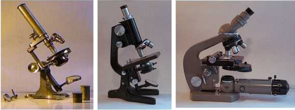
Three basic designs of microscope stand of the past 150 years.
