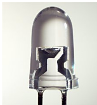
Narrow-beam white LED. ..with small source.
